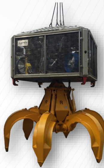
Above is the AUXROV shown with a 6 Tine grab and below is the clam shell grab.
