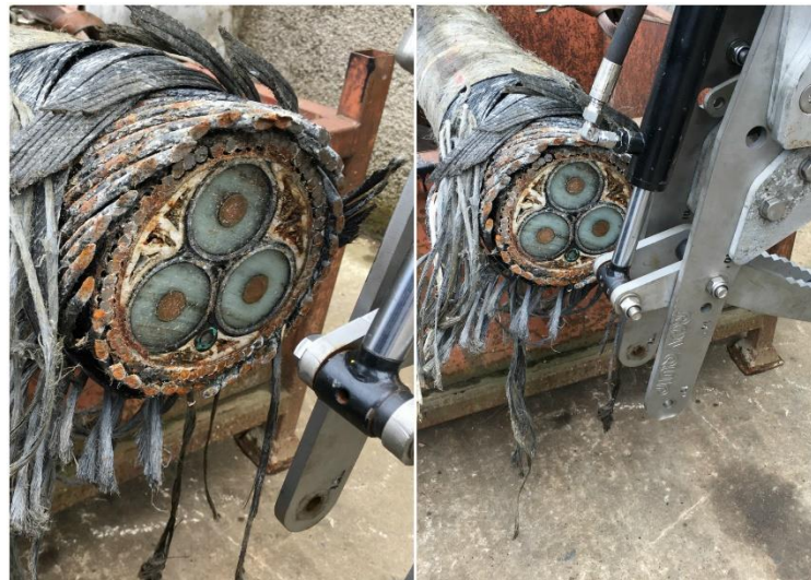
Picture above shows a test cut of 240mm multi layered armoured umbilical
